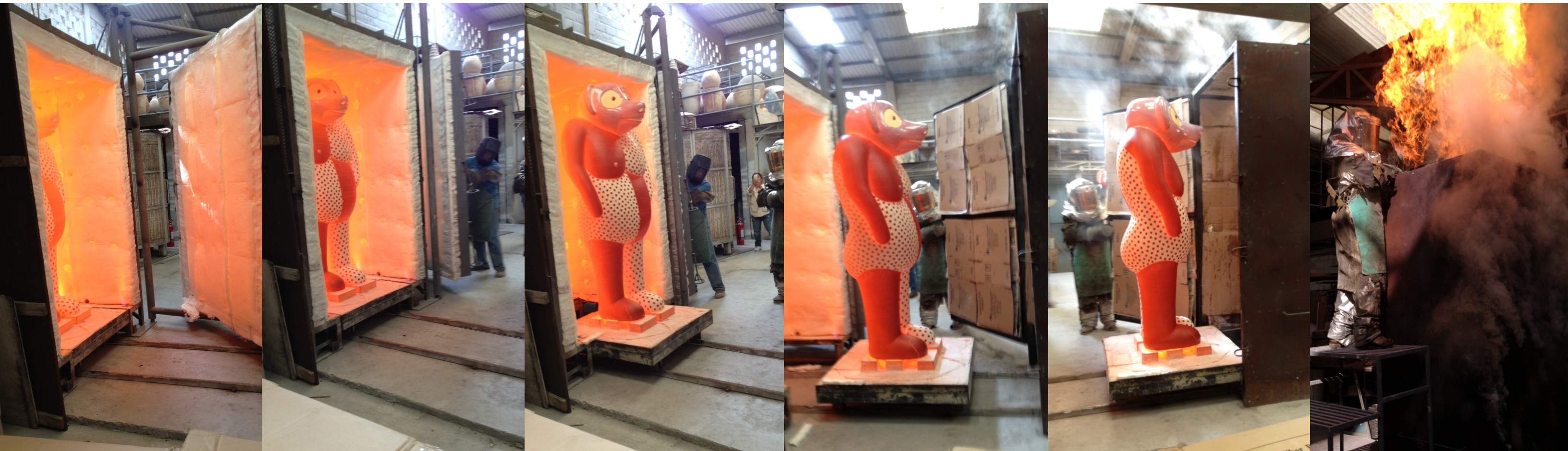
A glowing hot Tanuki exiting the kiln and being enclosed in a chamber lined with combustible materials
